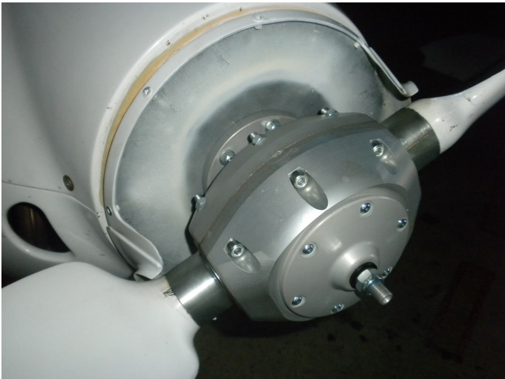
Picture no. 17 Propeller installation onto the propeller boss
