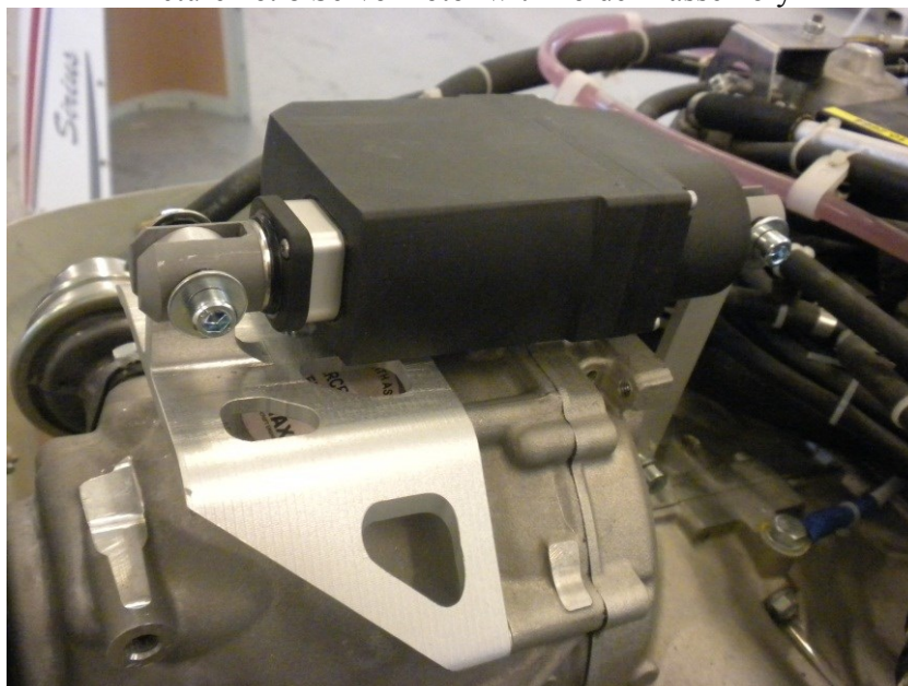
Picture no. 8 Servo motor with holder - assembly
