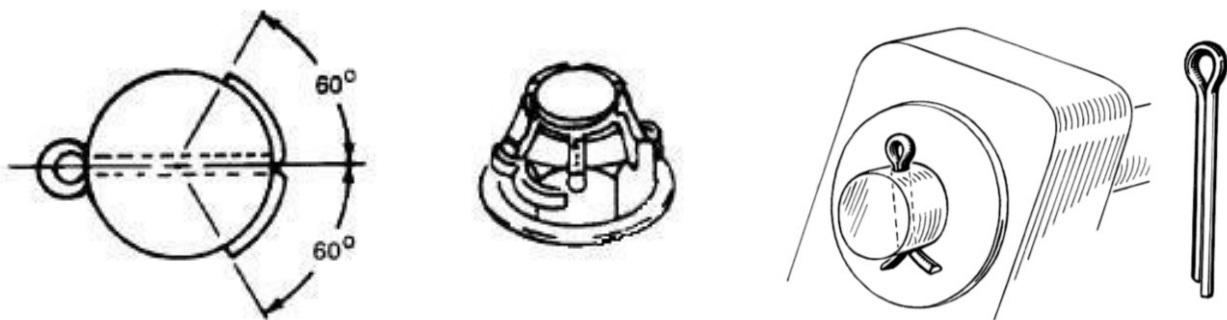
Figure: Securing bolts or castle nuts with a cotter pin.
